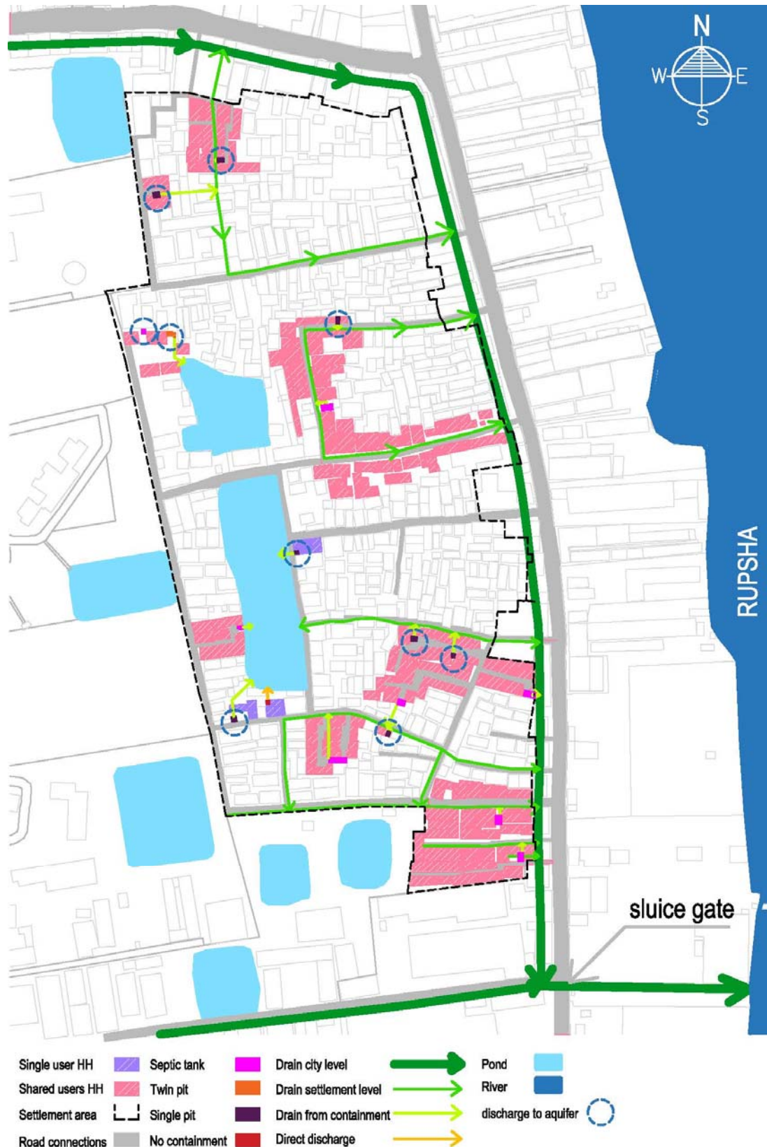
Figure 4.16: map of periodic FS discharge through pipe from sample containments, Source: author
